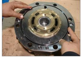
(9) Install casing (1) into assembling jig.
