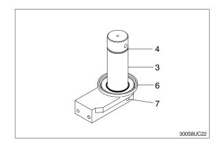
4 Install seal (5) to shell (1) and bracket (6).
