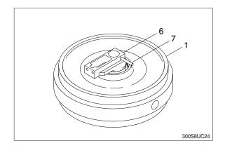
⑧ Lay bracket (6) on its side. Supply engine oil to the specified level, and tighten plug.
