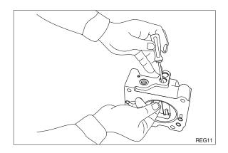
(8) Fit fulcrum plug (614) so that pin forcefitted in fulcrum plug(614) can be put into pin hole of lever (2).
