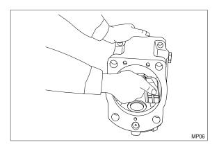
(12) Tapping lightly shaft's end of drive shafts(111, 113) with plastic hammer, take out drive shafts from swash plate supports.
