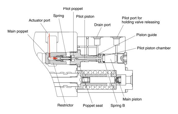
HOLDING VALVE BLOCK SECTION
