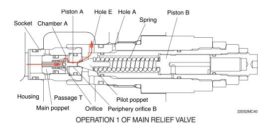
② The pressure in chamber A is lowered by moving of the pilot poppet and the main poppet is opened. As a result, the pressurized oil flows out to the tank passage through the hole of the socket side.
