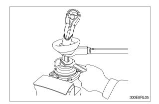
(17) Apply grease to rotating section of joint and contacting faces of disk and push rod.
