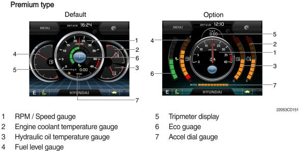
※ Operation screen type can be set by the screen type menu of the display (premium type). Refer to page 5-76 for details.
