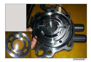
② Using a torque wrench, disassemble relief valve (30) from valve casing (23).
