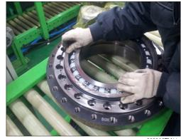
② Release 25 hex wrench bolts (28. M18) and remove ring gear (1) from housing (7).
