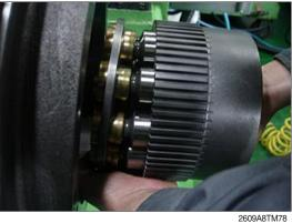
(22) Assemble separated plate (24), friction plate (23) into cylinder block in regular sequence. Friction plate : 4EA Separated plate : 5EA
