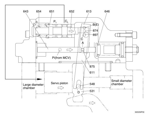
As the pilot pressure Pi rises, the pilot piston (643) moves to the right to a position where the force of the pilot spring (646) balances with the hydraulic force.
