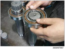
(11) Assemble the heated needle bearing inner ring on the shaft (8).
