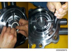
⑥ Apply some grease valve plate (20) and assemble it into valve casing (23).
