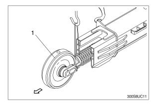
(3) Remove the bolts (2), washers (3) and separate idler from recoil spring.
