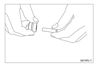
(13) Remove O-ring (10) and seal (11) from plug (8).Use small minus screwdriver or so on to remove this seal.
