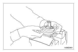
(13) Fit boot (23) and lock nut (22), and handle subassembly is assembled completely.
