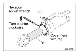
④ Draw out cylinder head and rod assembly together from tube assembly
