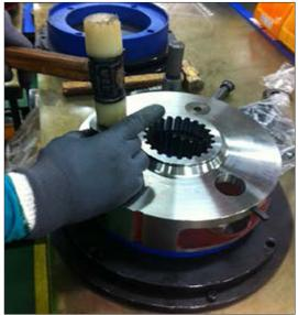
2 Assemble spring pin No.1 (25) to fix carrier No.1 (20) and spring pin No.1 (25) by using the jig.
