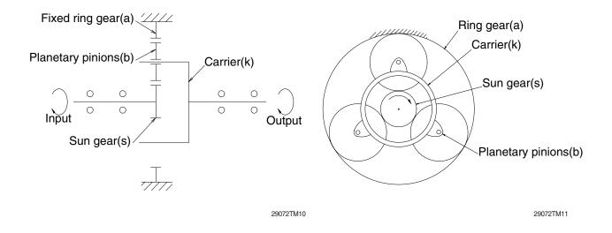
When the sun gear S1 is driven by input shaft, planetary action occurs among gears S1, a and b and revolution of gear b transfers the rotation of carrier K1 to second sun gear S2, and also evokes planetary action between gear S2, a and d.
