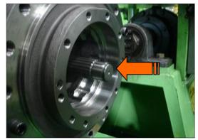
(15) Disassemble valve plate (28) into rear cover (34).
