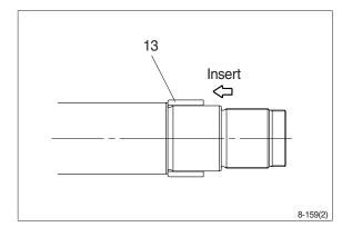
(5) Fit piston assembly to rod assembly.  $\cdot$  Tightening torque : 100±10.0 kgf  $\cdot$  m (723±72.3 lbf  $\cdot$  ft)
