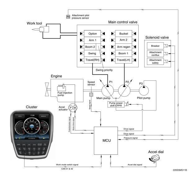
• The system is used to control the pump delivery flow according to set of the work tool on the cluster by the attachment flow EPPR valve.
